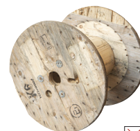
Outer plank missing MAX 2 planks are repairable
