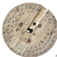
Inner plank on flange missing
